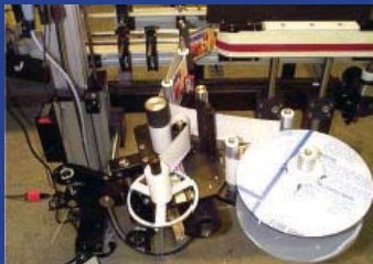
Utility labelling head and the wrap station of the Basic WrapAround (BWA) system
